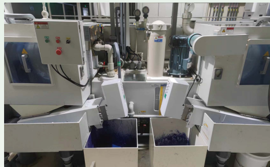
Online dry film residue reduction equipment
