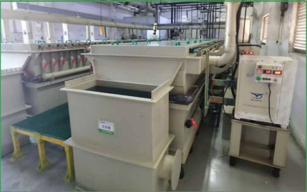
Recovery of copper in etching waste solution by electrolysis, reducing copper-containing waste solution.
